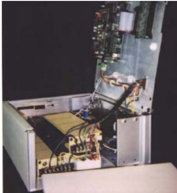
Figure 5. Inside view of the electronics box of LabRAT 1 showing power supplies and signal processing boards.
