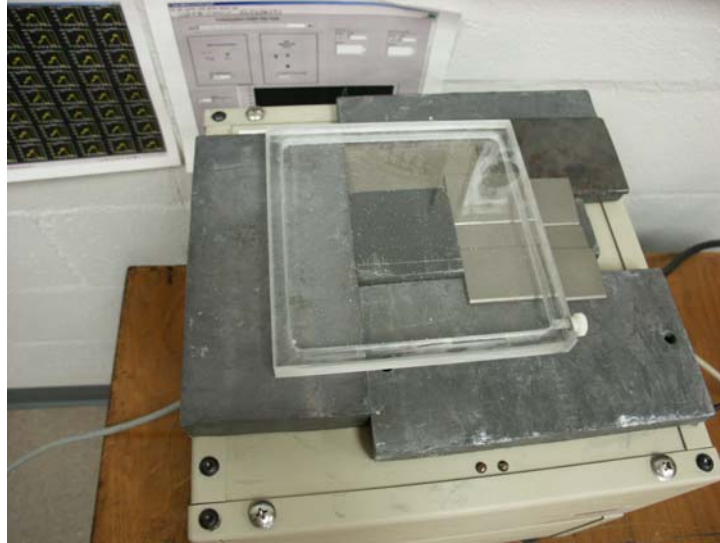
Figure 54. Photograph of setup for extrinsic uniformity test including parallel hole collimator in the center, lead shielding around the collimator and the water tank phantom.
