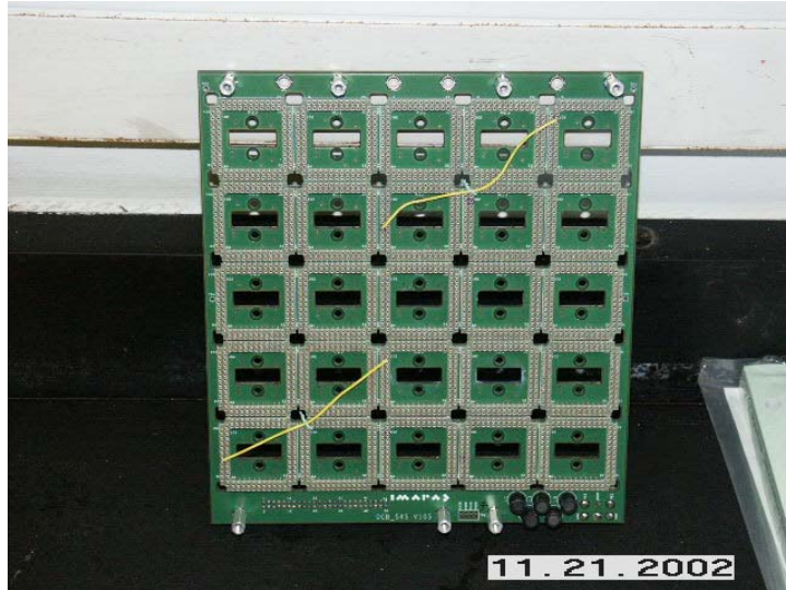
Figure 8. Photograph of the carrier board used in the LabRAT systems. The carrier board holds up to twenty-five CZT modules.
