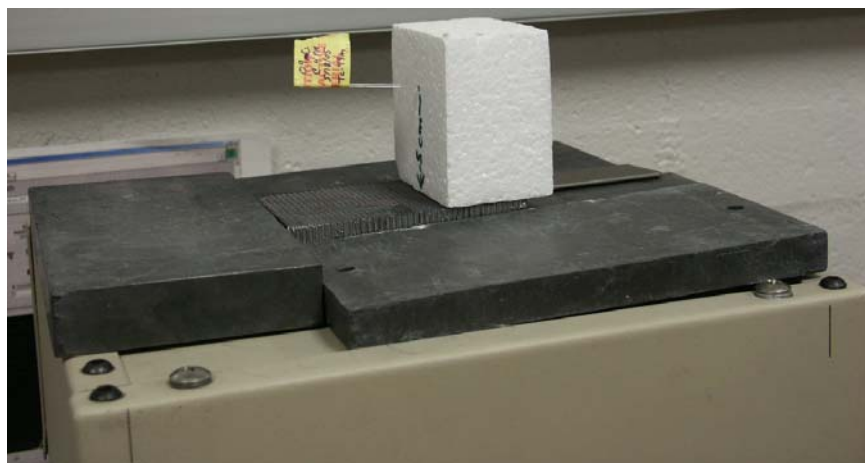
Figure 44. Photograph of experimental setup for measuring extrinsic spatial resolution. The capillary tube is positioned parallel to and 5 cm above the collimator face. Lead sheet around the collimator provides lateral shielding.
