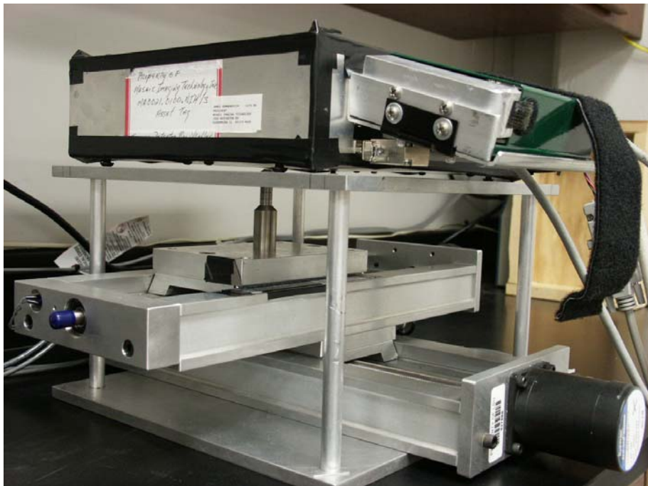
Figure 33. Point source scanning system with detector frame and point source holder. LabRAT 0 is in place on the frame.
