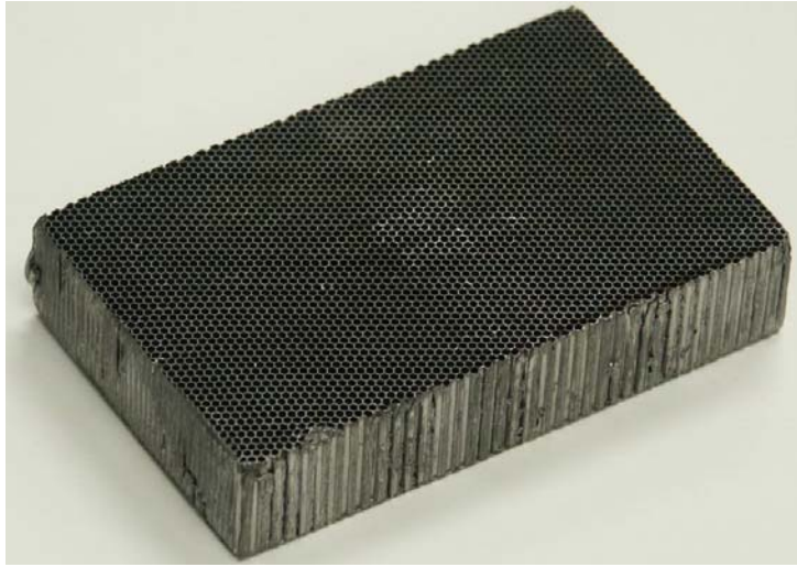
Figure 45. Photograph of the low-energy, all-purpose collimator used for extrinsic spatial resolution and uniformity measurements. This piece of collimator is a lead-foil, hexagonal hole design from a Siemens' LEAP collimator.
