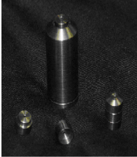
Figure 32. Tungsten source holder and collimator discs used for spatial resolution and uniformity of response measurements.
